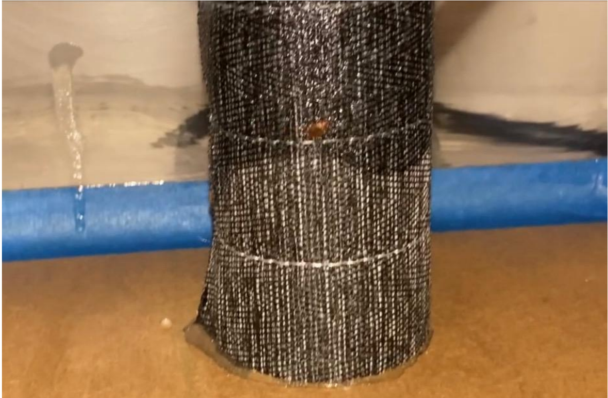
Figure 4. One adult bed bug attempting to climb up the double-coated Averzion Slick barrier.
