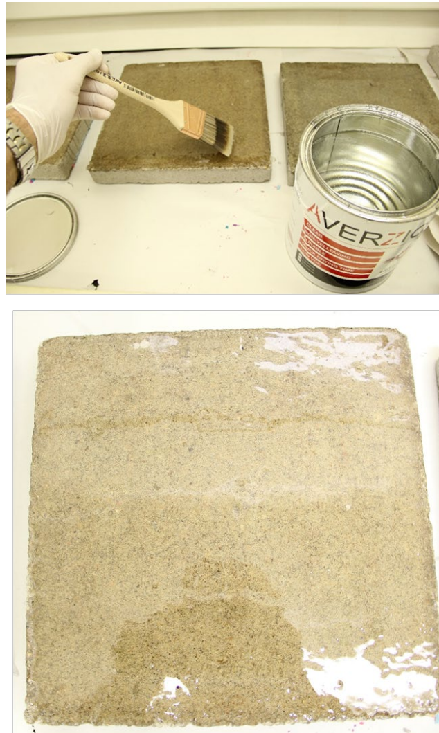
Figure 3. Slabs painted with Averzion. Three coats were put to achieve a smooth surface.
